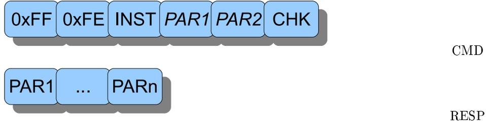
Figure 4. Command and Response Packets of HaViMo2.5.
